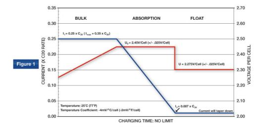
The initial charge current is recommended to be set at I = 0.25 X C (Im = 0.35 X C) in order to fully charge the batteries within a reasonable amount of time. It can be set lower, however please be aware that charge time will increase so make sure the batteries have enough time to fully charge before being put back into service Fullriver batteries have a low internal resistance allowing them to be charged at a higher current, therefore faster, than conventional flooded/wet batteries.
