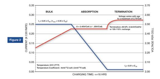
$\label{eq:bulk-stage-Set} \text{Bulk stage - Set the charger to the initial current I until the voltage limit U is reached.}$
